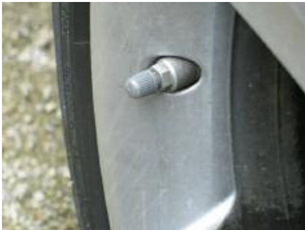
"Threaded" Valve stem on vehicles which monitor actual tire pressure.
